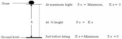
**Note that**: Potential energy decreases from maximum to zero and the kinetic energy increases to maximum. This is because as the h value decreases to zero, the velocity increases to maximum.
