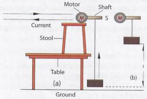
If the mass is lifted through a distance, h, in a time t, as shown in figure (b) above, then, Power of the motor  $=\frac{Workdone}{Time} = \frac{Mass of body (m) \times g \times height(h)}{t}$ Knowing the mass, m, of the body, the time taken, t, to lift the mass through a height h, the approximated power of the motor can be calculated.
