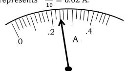
The illustration above shows an ammeter reading =  $(12 \times 0.02) = 0.24$  A. Ammeter readings are written up to 2 decimal places and occur in multiples of 2.
