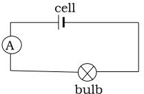
This ensures that the current that passes through the device is the same current that passes through the ammeter.
