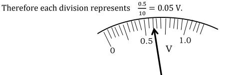
The illustration above shows a voltmeter reading =  $(12 \times 0.05) = 0.60$  V.
