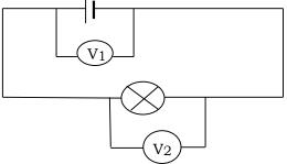
Voltmeter  $V_1$  measures the p.d between the terminals of the cell, while  $V_2$  measures the p.d across the bulb.
