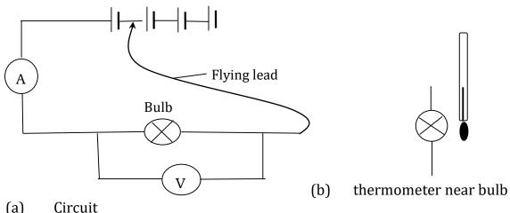
The thermometer will show an increase in temperature. When the thermometer has attained a steady reading then the ammeter reading (I), voltmeter reading (V) and thermometer reading,  $\Theta^{\circ}$  C are recorded in a table.
