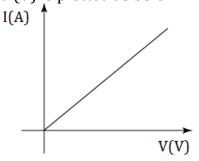
The graph is a straight line passing through the origin. This shows that *the current is directly proportional to the applied potential differential*.
