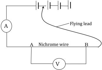
The circuit is connected as shown in the diagram above. The ammeter and voltmeter readings are recorded.
