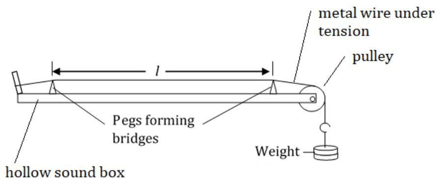
This is an instrument used for studying behavior of vibrating strings.
