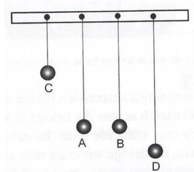
Four pendulum points A, B, C and D are suspended from a light wooden metre rule fairly well-damped at its ends. A and B are made of the same length, C shorter and D longer. A is set into oscillations, in a plane perpendicular to the plane containing the pendulums.
