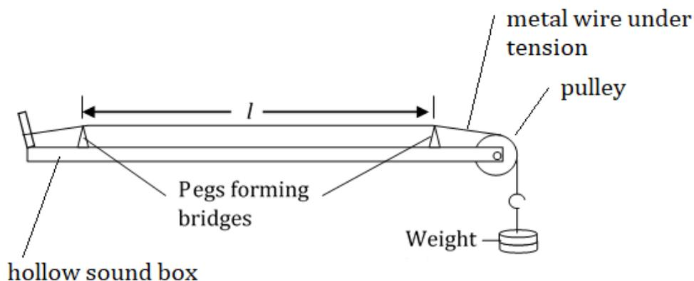
A tuning fork of known frequency is set into vibrations and the stem of the vibrating tuning fork is gently pressed on the sonometer box. The tuning fork in the vibrating state “forces” the box to vibrate, the vibrations are transmitted through the box to the wire.
