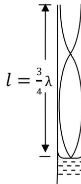
If the water level is lowered further, another point is reached lower down for which resonance again occurs. The air column =  $\frac{3}{4}\lambda$
