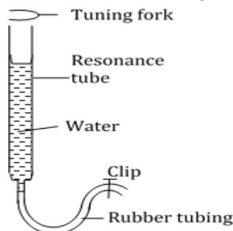
The resonance tube is first filled with water
