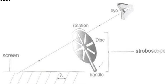
It is a disc with equally spaced slits which can be rotated by hand or a motor.
