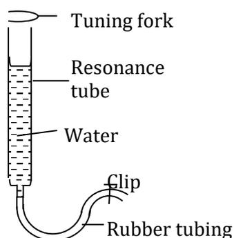
A resonance tube is almost filled with water
