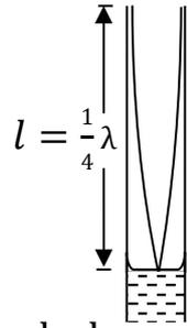
Sound from the tuning fork travels down and is reflected by the water surface and a stationary wave is formed of a node corresponds to the water level.
