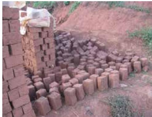
*Fig. 2.2a: Bricks made from soil*
